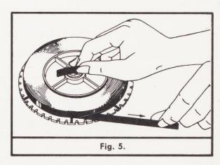
12. Splice tape in normal manner. Read note below before splicing. Use Mylar base splicing tape if available. Acetate base splicing tape will generally break after approximately 100 hours of operation on a fully loaded cartridge.
