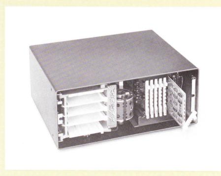
The six printed circuit cards contain the read/write and controller electronics and power regulation circuitry. The card ejector lever on each card also exposes six test points for ease of servicing. An extender card is stored in the cabinet to the right of the card cage.
