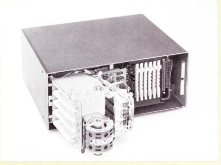
The entire transport assembly pivots outward for access to tape drive components, magnetic heads, and transport control electronics, all of which are mounted on the one-piece transport casting. The mechanical simplicity of a single motor, single capstan, and individual tape drive actuators insure the reliable operation for which CartriFile tape systems are well known.
