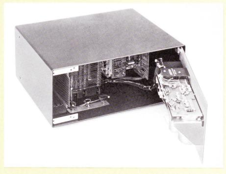
The power supply assembly swings outward from the rear of the wrap-around cabinet. The brackets on the left mount the connector (not shown) which carries data and control signals between the CartriFile 40 and the computer. Even from the rear, the uncluttered, good design and workmanship of the CartriFile 40 are apparent.
